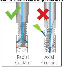
**Chip Evacuation in Thru Holes using Axial & Radial Coolant**
